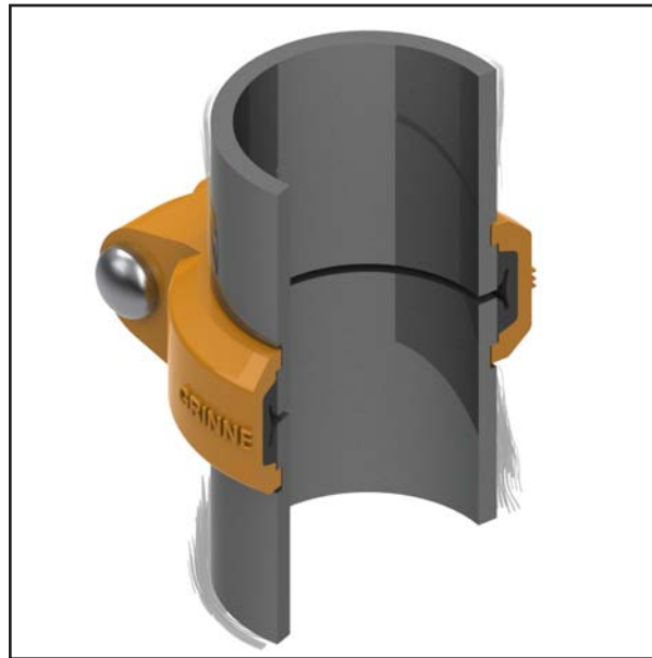
Figure 1: Section view of a GRINNELL Grooved Coupling
