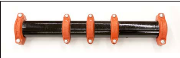
Figure 7: The Three Different Pipe Assembly Joints Tested for Vibration Attenuation
